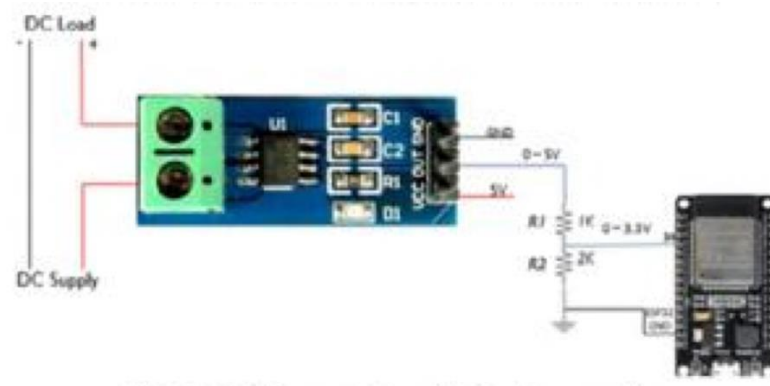
Gambar 4.4. Koneksi ACS712 ke mikrokontroler ESP32. (Sumber : Low-Cost Open Source IoT-Based SCADA System for a BTS Site Using ESP32 and Arduino IoT Cloud, 2021)
